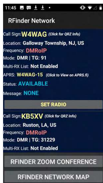
Figure 5 — The RFinder on the Air feature, showing who is available on the network in real time.
